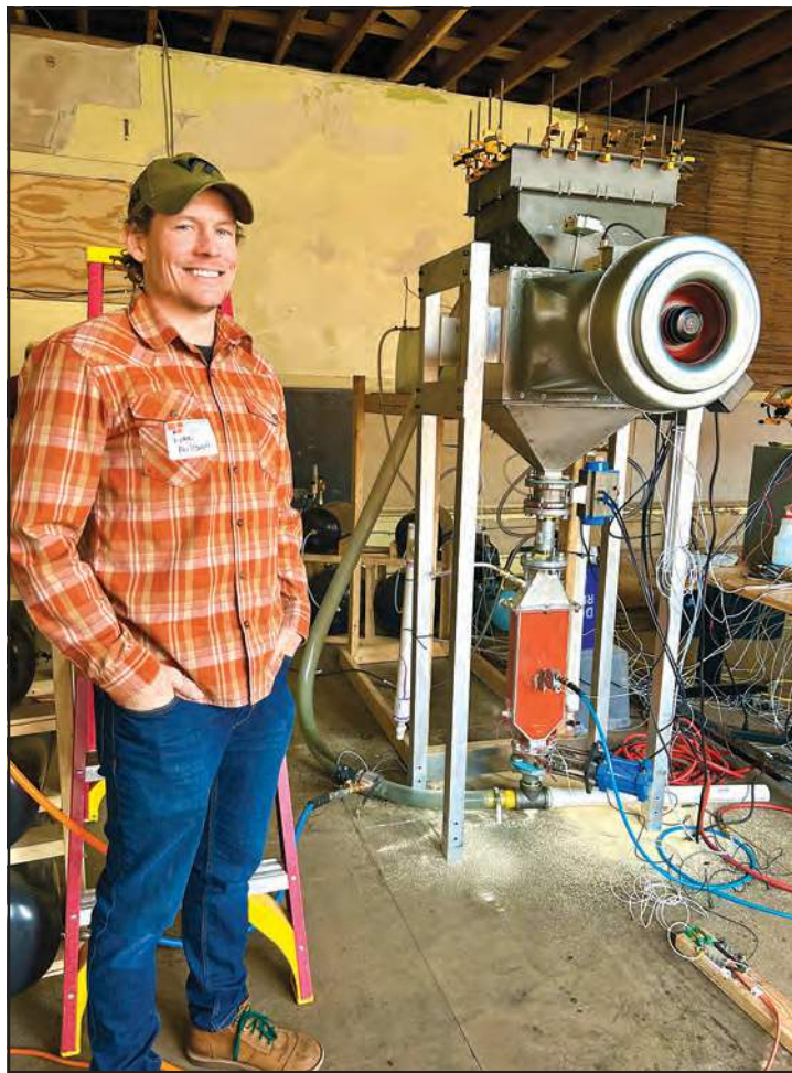
Luke Allison, Chief Development Officer for Vegg Inc. stands next to the patented Direct Air Technology developed by MOVA to extract CO 2 from the atmosphere.
